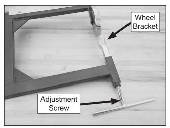
**Figure 6.** Lower wheel adjustment screw installed.
